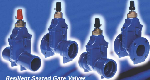
Resilient Seated Gate Valves For below ground (sluice) DN80 - DN600. Class 16. Flanged DN100 - DN375. Class 16. Socketted DN80 - DN375. Class 16. Spigotted
