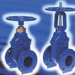
Resilient Seated Gate Valves For above ground Rising Spindle (OS&Y) & Non-Rising Spindle. DN80 - DN300. Class 16. Flanged
