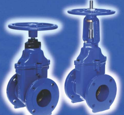
Metal Seated Gate Valves For above ground Rising Spindle (OS&Y) & Non-Rising Spindle. DN80 - DN300. Class 16. Flanged
